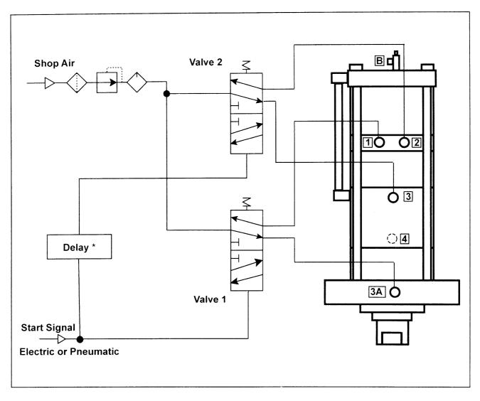
\* DELAY: The Power Stroke (High Pressure) can be initiated in many ways, including time delay, pressure build up, pressure decay or position sensing.
